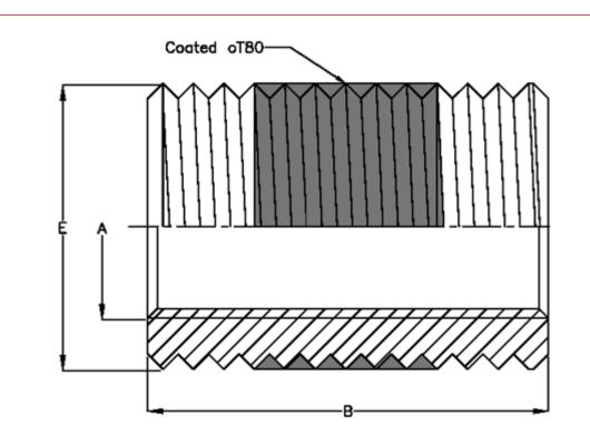
Female thread A = M3Length B= 6Male thread E= M5Type= 97x 000 030.100
